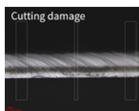
Figure 5. Cell cutting damage
