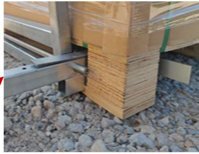
“L” shape lock on the pallet foot
